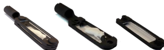
Animal holders for hybrid FLT/CT and BLT/CT imaging.
